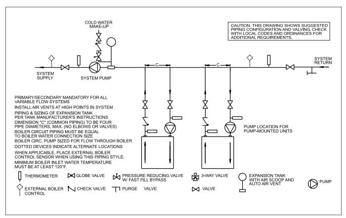
Figure 4. Hydronic Piping — Multiple Boilers, Primary Secondary System.
